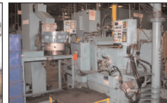
NIPPEI TOYAMA CORP (NTC) MODEL CLG-3BN CNC TWIN GRIP CENTERLESS THROUGH FEED GRINDER
