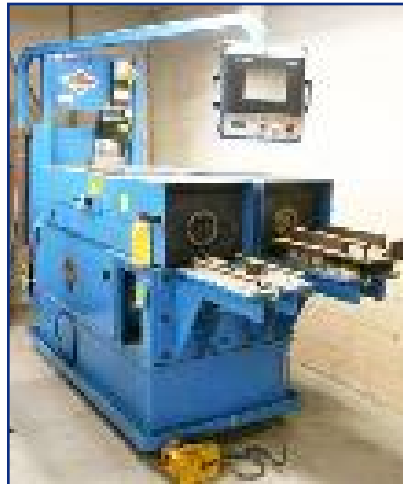
MCKEE-ADDISON MODEL FORMASTER 70 ID/OD + ID/OD DUAL SIZER HORIZONTAL HYDRAULIC TUBE END FORMING MACHINE
