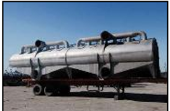
SAMPLE VIEW OF THE TYPE OF VOITH FLOTATION CELL USED IN THIS FACILITY
