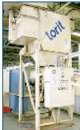
(1 OF 2) TORIT DONALDSON DF-2DF8 DUST COLLECTORS
