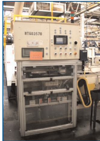
(1 OF 2) ZERSTORUNGSFREIE EDDY LINER P4 PMFT (PREVENTATIVE MULTI FREQUENCY TEST) EDDY CURRENT TEST STANDS
